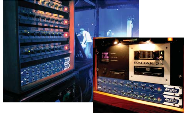
Thirty-two channels of line-level input on stage (left), using existing mic preamps, and a 24-channel split to remote recording (right).
