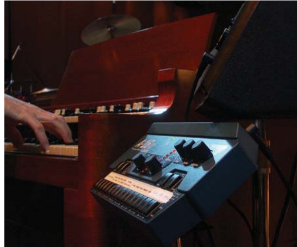
Aviom's A-16II personal mixer allows every performer to customize his own mix, without affecting other monitor mixes, the front-of-house mix, or recording/broadcast feeds.
